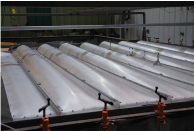
▲ An ASTM E 1592 test bed showing a 16-inch horizontal seam panel system pressurized to 126 psf using S-5 WindClamps™ at panel clip locations. The assembly failed at 220 psf. The failure pressure without seam reinforcement was 110 psf.
