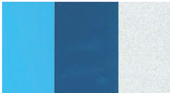
▲ A Megaflon (100 percent FEVE) blue, 70 percent PVDF blue and 70 percent PVDF silver metallic finish. Image courtesy of PPG Industries, Pittsburgh, PA.
