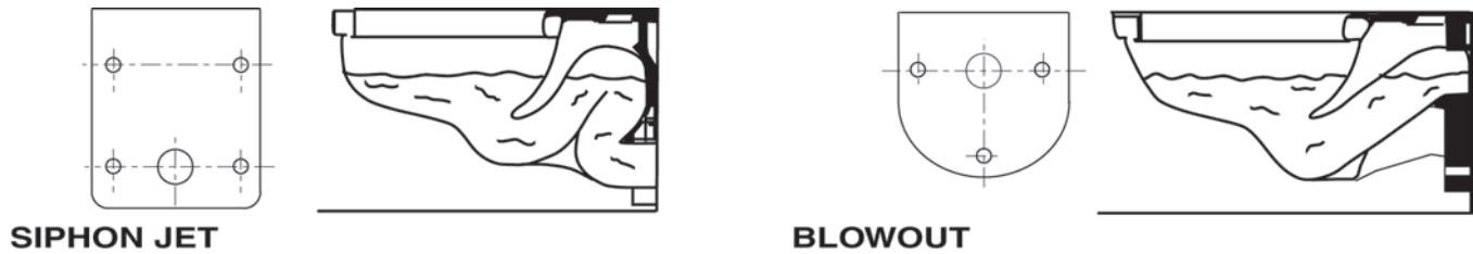
Figure 3. Water Closets: Types and Support Structures.
